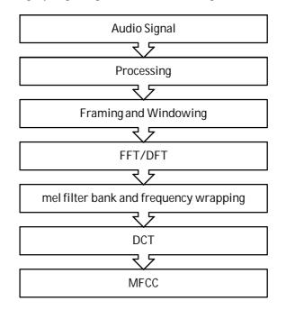
Fig 1. Step by Step Computation of MFCC
